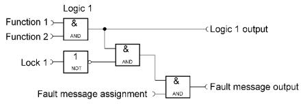
All logic and timer functions can be assigned to the fault message groups and to the collective fault. The available blocking functions are also available for all logic and timer functions. Each input function is invertible.
