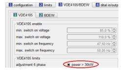
For systems with more than 30 kVA, the corresponding value must be activated in the parameterisation (*figured left*). The voltage monitoring then takes place both at the star-point voltage and at the external connector voltage.
